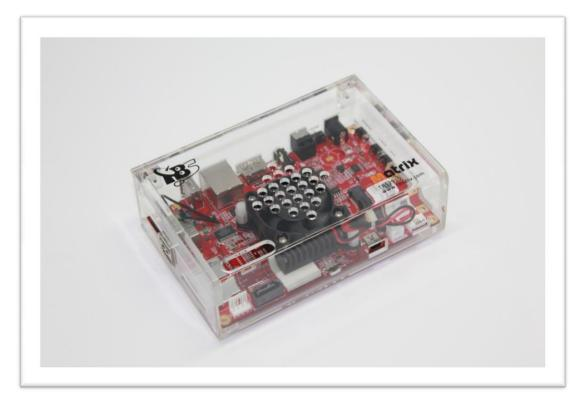
**Matrix** is a single board mini computer based on ARM with a wide range of interface, equipped with a powerful i.MX6 Freescale processor, it can run Android, Linux and other operating systems, a switch between different operating systems can be done within just a few minutes! Matrix also has great support for TBS USB tuners and popular software such as XBMC, VDR, Tvheadend, DVBLast and so on.
